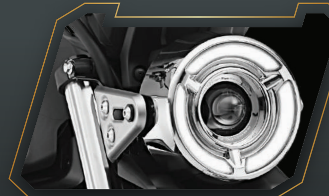
BI-FUNCTIONAL LED HEADLIGHT WITH DRL
